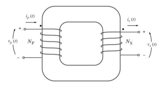
The voltage equations for a single-phase transformer with a primary winding "p" and secondary winding "s", and voltages  $v_p$  and  $v_s$ , can be expressed as follows:
