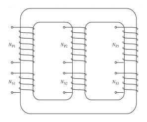
$$\lambda_{p1} = L_{p1p1} * i_{p1} + L_{p1p2} * i_{p2} + L_{p1p3} * i_{p3} + L_{p1s1} * i_{s1} + L_{p1s2} * i_{s2} + L_{p1s3} * i_{s3}$$
