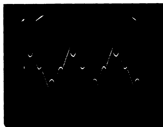
Figure (7): OSCILLOGRAM OF MACHINE PHASE CURRENT, TEST #1: ROTOR SPEED=1750 r/min. (Horizontal: 5ms/div. Vertical 1 A/div.), 1.7 A peak
